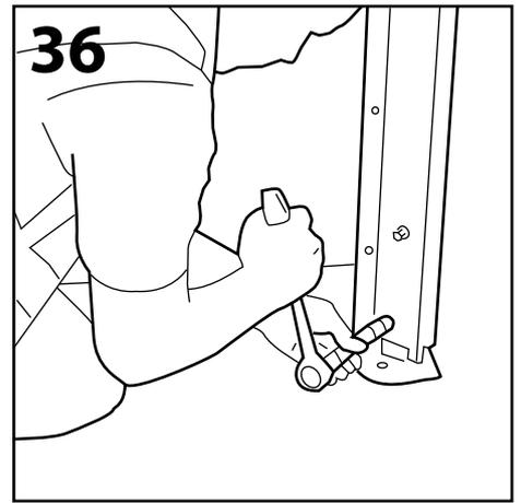
Replace the bolts and washers into the new holes within the spigot leg and tighten with spanner/socket. Repeat Figs 34-36 on the other legs that need adjusting.
